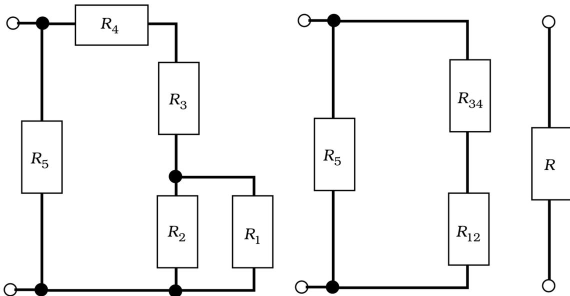
$$\frac{1}{R_{12}} = \frac{1}{R_1} + \frac{1}{R_2} \quad \rightarrow \quad R_{12} = \frac{R_1 R_2}{R_1 + R_2}$$
